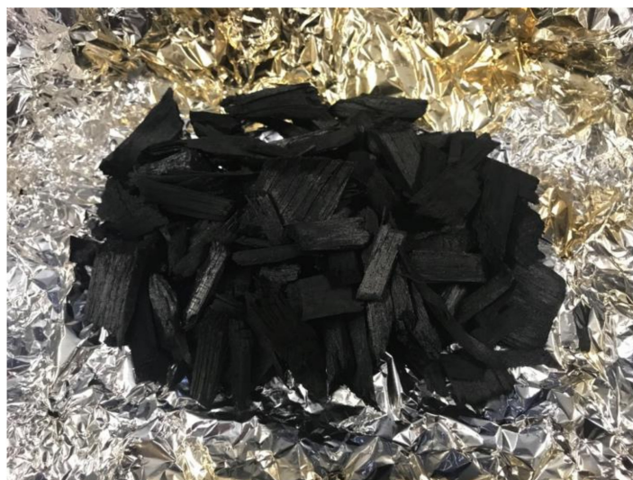
Figure 3. Example of one of the obtained materials, in this case torrefied pine woodchips.
