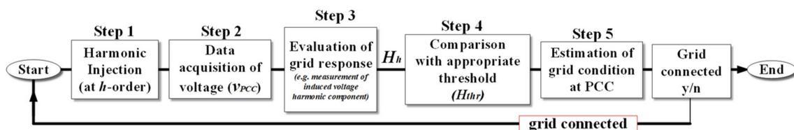
**Figure 1.** Generic description of the harmonic injection based anti-islanding techniques.
