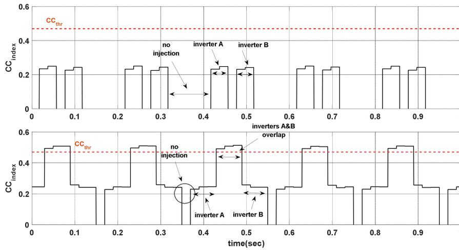
**Figure 11.** Evolution of  $CC_{index}$  in an islanded operation for the two injection patterns, (top graph) 1/10 cycles, (bottom graph) 6/10 cycles.
