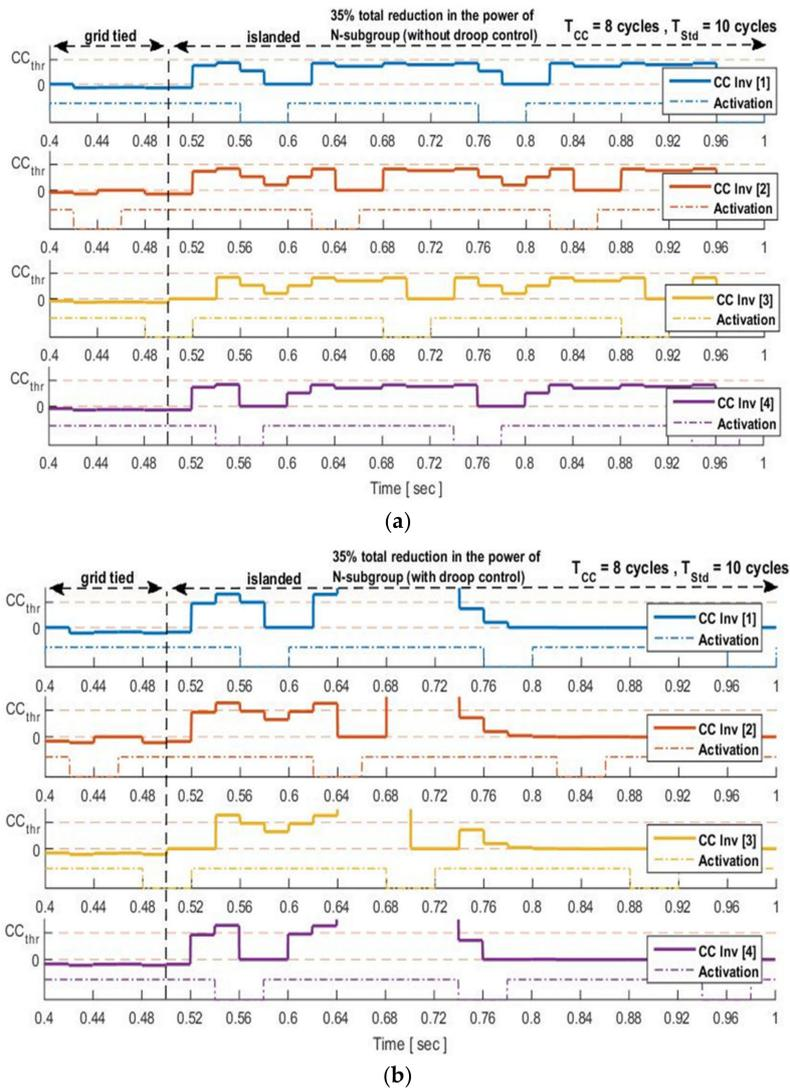
Figure 9.  $CC_{index}$  of inverters under reduced power operation (60% and 80% reduction for the inverters 2 and 3, respectively) for  $l = 4$  ( $T_{CC} = 8$  cycles), (a) without droop-controller, (b) with droop-controller.
