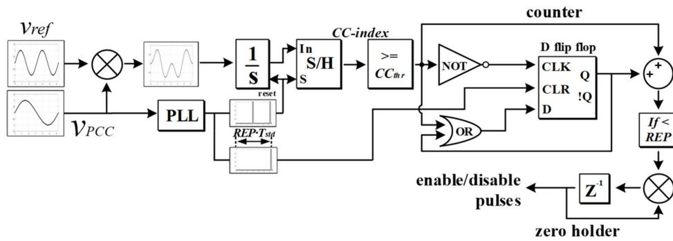
Figure 4. The anti-islanding technique that has been proposed in reference [2].
