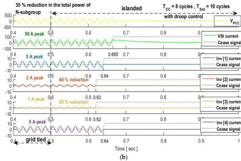
**Figure 10.** PCC voltage and inverter currents at reduced power levels (60% and 80% reduction for the inverters 2 and 3, respectively) and  $l = 4$  ( $T_{CC} = 8$  cycles), (a) without a droop-controller; (b) with a droop-controller.
