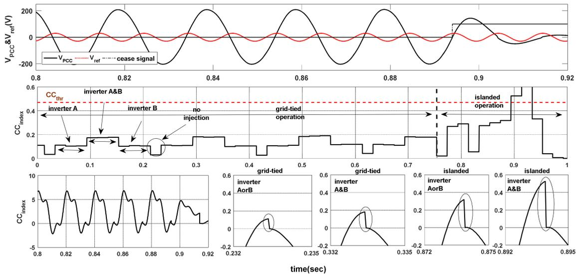
**Figure 12.** (top graph)  $V_{PCC}$  along with  $V_{ref}$ , (middle graph) evolution of  $CC_{index}$  in grid tied and islanded operation, (bottom graph) evolution of the  $CC_{index}$  calculation.
