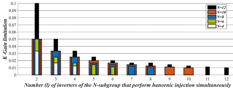
Figure 7.  $K$ -Gain limitation as a function of  $l$ , for five indicative  $N$ -values (i.e.,  $N = 4, 6, 8, 10, 12$ ).
