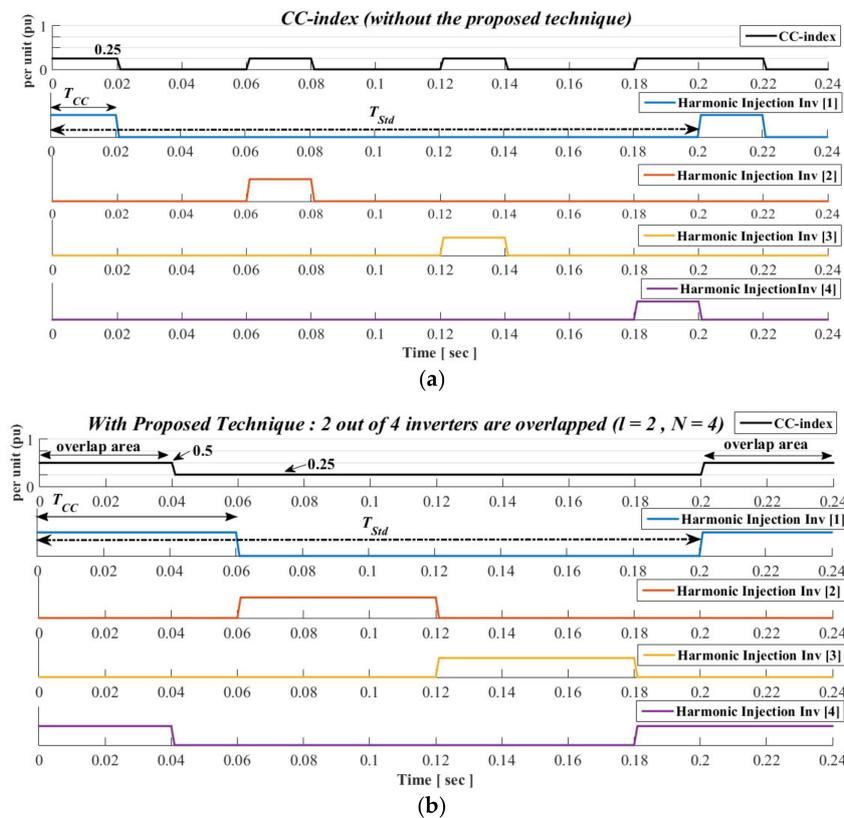
**Figure 5.** Injection pattern of the  $N$ -subgroup inverters and  $CC_{index}$  evolution in a time domain for, (a)  $N = 4$  and  $l = 1$ , (b)  $N = 4$  and  $l = 2$  (implying that at least two inverters will be overlapped).
