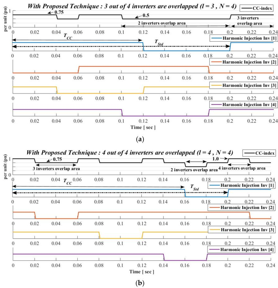
**Figure 6.** Injection pattern of the  $N$ -subgroup inverters and  $CC_{index}$  evolution in a time domain for, (a)  $N = 4$  and  $l = 3$  (implying that at least three inverters will be overlapped), (b)  $N = 4$  and  $l = 4$  (implying that at least four inverters will be overlapped).
