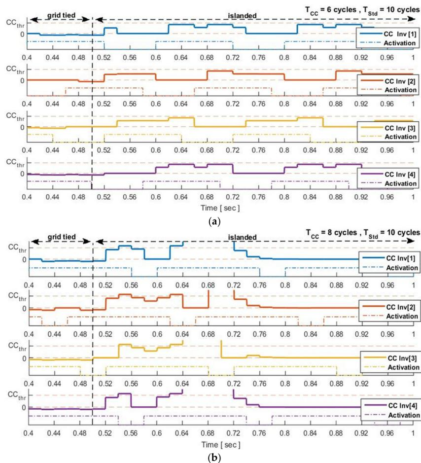
**Figure 8.**  $CC_{index}$  of inverters under nominal power operation, (a)  $l = 3$  ( $T_{CC} =$  six cycles), (b)  $l = 4$  ( $T_{CC} =$  eight cycles).
