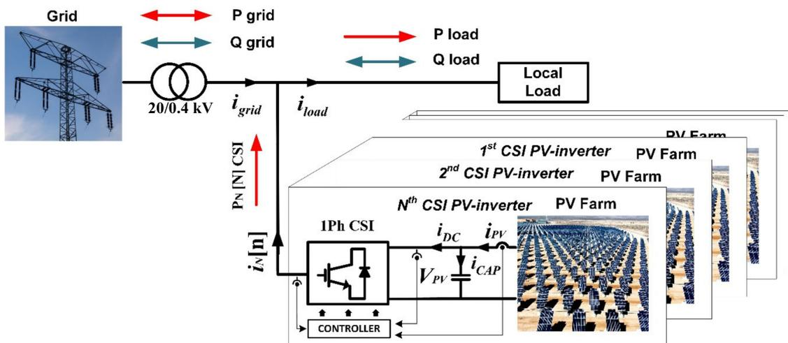
Figure 2. Schematic diagram of the system under study, where PV-distributed energy resources (DER) generators have been used.
