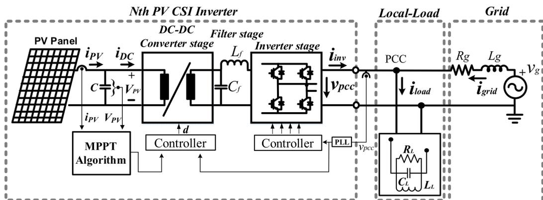
Figure 3. Electrical diagram of a PV-based DER-CSI.
