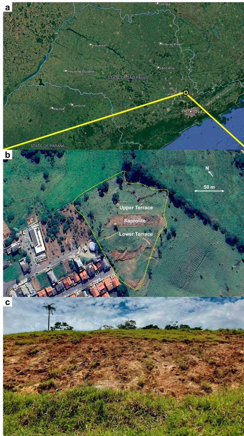
**Figure 1.** Satellite photographs showing (a) the location of the Morungaba study site within the state of São Paulo, and (b) the outer perimeter of the study site, with the positions of the upper terrace, lower terrace, and saprolite slope indicated. Photograph (c) depicts the saprolite slope studied in this paper, as seen from the lower terrace.
