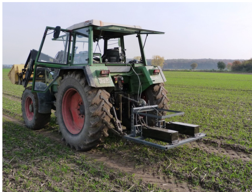
Figure 1. Set-up for recording gamma spectra stop-and-go as well as on-the-go. The two crystals mounted to the steel frame are positioned 0.3 m above the soil surface. The photomultiplier console and the computer are in the tractor cabin.
