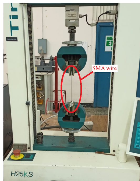
Figure 3. Hysteresis tensile testing of SMA wire using a Tinius Olsen Universal Tester.
