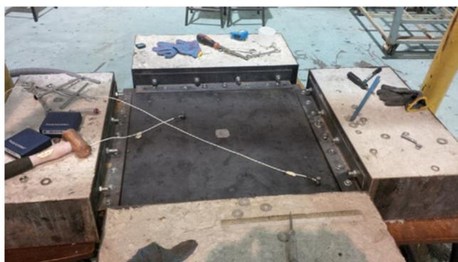
Figure 12. A fully clamped steel plate with middle damage [81].
