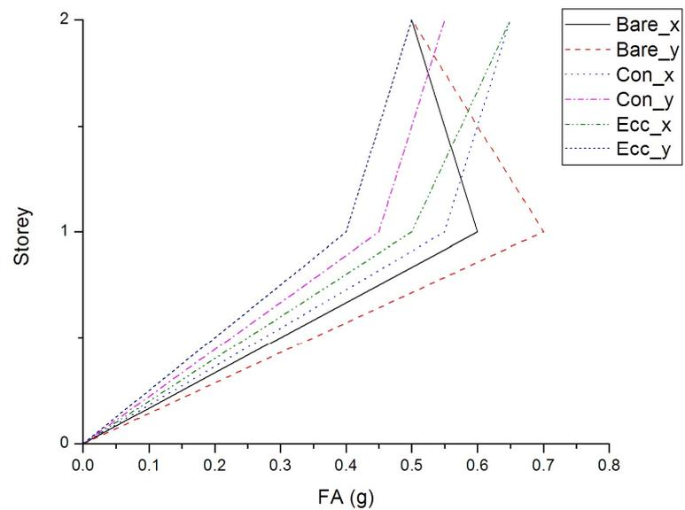
**Figure 6.** Distribution of peak FA for the RC building with and without the seesaw system, subjected to seismic motion No. 4 of Table 3.
