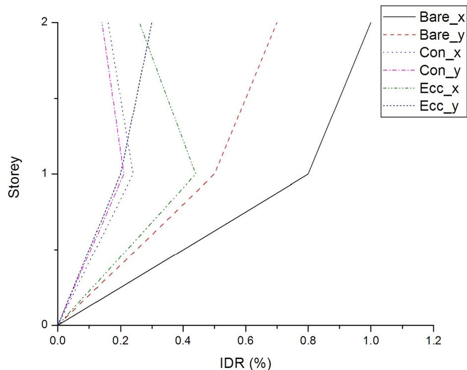
**Figure 4.** Distribution of peak IDR for the RC building with and without the seesaw system, when subjected to seismic motion No. 4 of Table 3.
