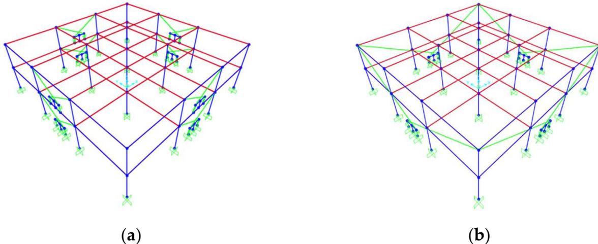
**Figure 3.** Concentric (a) and eccentric (b) installation of the seesaw system in the two-storey RC building.
