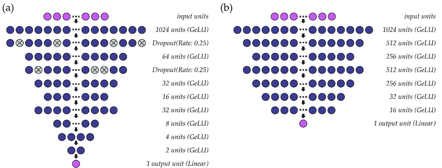
**Figure 3.** Structure of the multi-speaker deep regression neural networks used to estimate (a)  $f_0$  and (b) intensity from sEMG signals.
