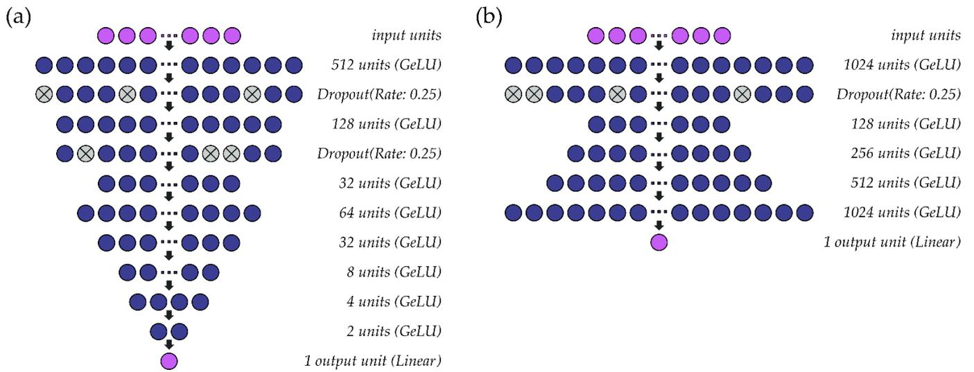
**Figure 2.** Structure of the single-speaker deep regression neural networks used to estimate (a)  $f_0$  and (b) intensity from sEMG signals.
