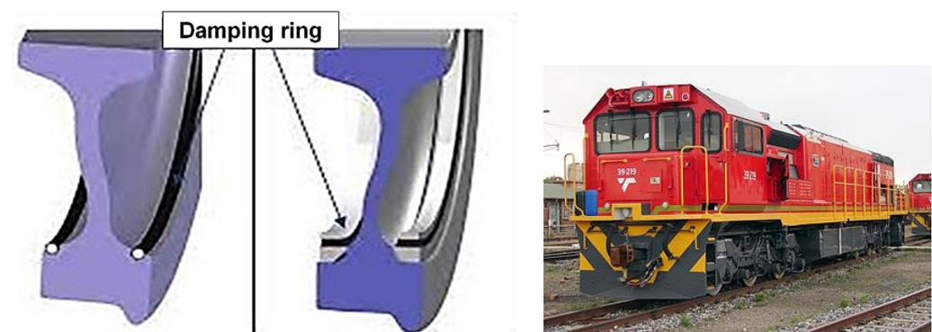
Figure 1. Damping ring under the rim of both sides of the wheel [19].
