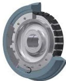
**Figure 3.** Locomotive wheel with resilient layer inserted between the hub and tread [28].
