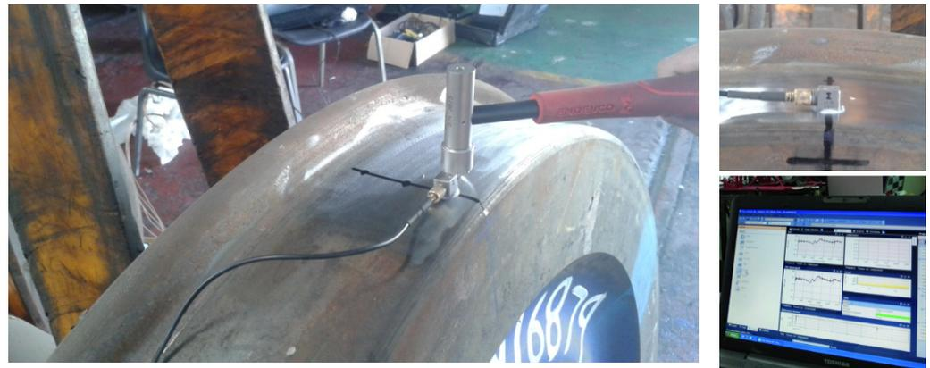
**Figure 4.** Experimental modal analysis (EMA) of D39200 locomotive wheel.
