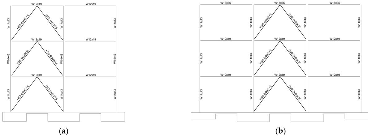
Figure 2. LFRS of test structure: (a) Braces along gridlines B and C, looking east (typical); (b) Braces along gridline 2, looking north.
