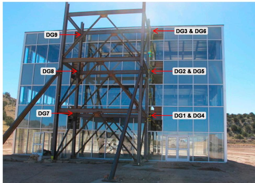
**Figure 7.** View of the instrumentation tower on the north (rear) elevation of the test structure indicating the locations of the displacement gauges (DG) at the three floor levels (same configuration on both tests).
