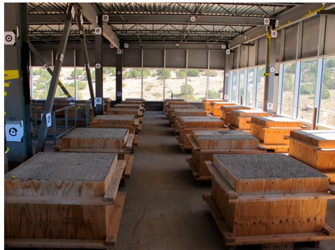
Figure 11. View of the concrete blocks for approximating loads under operational conditions consistent with extraordinary load combination of ASCE/SEI 7-10 [20] (45 per floor, 90 total on 2nd & 3rd floors).
