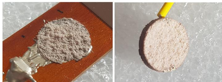
**Figure 5.** Test 9 which detached during the dynamic experiment.
