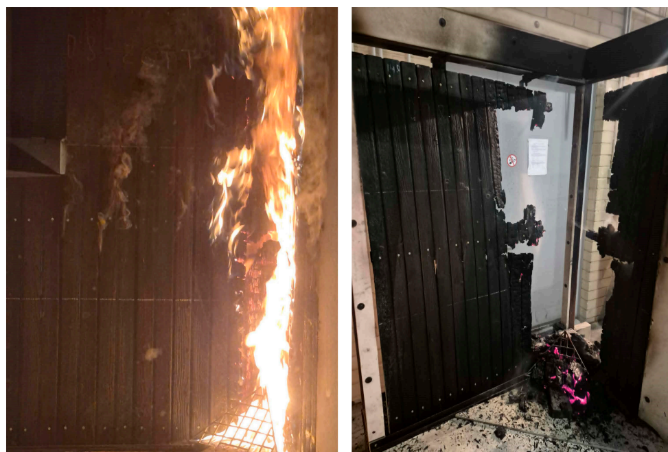
Figure 6. Image of samples during and after testing using the SBI method.
