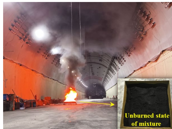
Figure 5. Combustion state of fire source.
