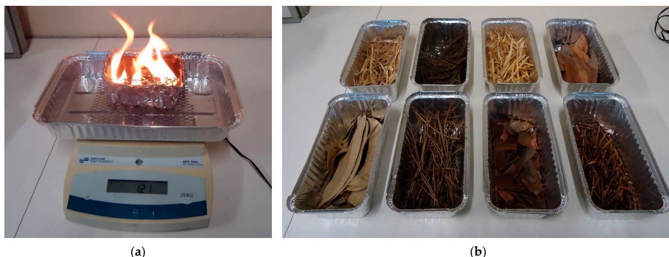
Figure 1. Experimental apparatus and fuel types: (a) combustion test using a fuel bed of Pinus pinaster needles; (b) fuel types: top row from left to right— Triticum spp. and Secale cereale leaves, Acacia dealbata leaves, Triticum spp. and S. cereale straw, and Eucalyptus obliqua leaves; bottom row from left to right— Eucalyptus globulus leaves, P. pinaster needles, E. globulus bark, and E. globulus twigs.
