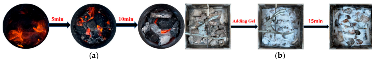
Figure 10. Effect of gel-covered coal combustion fire extinguishing; (a) Coal combustion process; (b) The thermosensitive hydrogel fire extinguishing effect.
