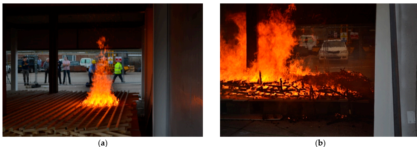
Figure 4. Fire development and travel: (a) early fire development (6 min); (b) fully developed travelling fire (32 min).
