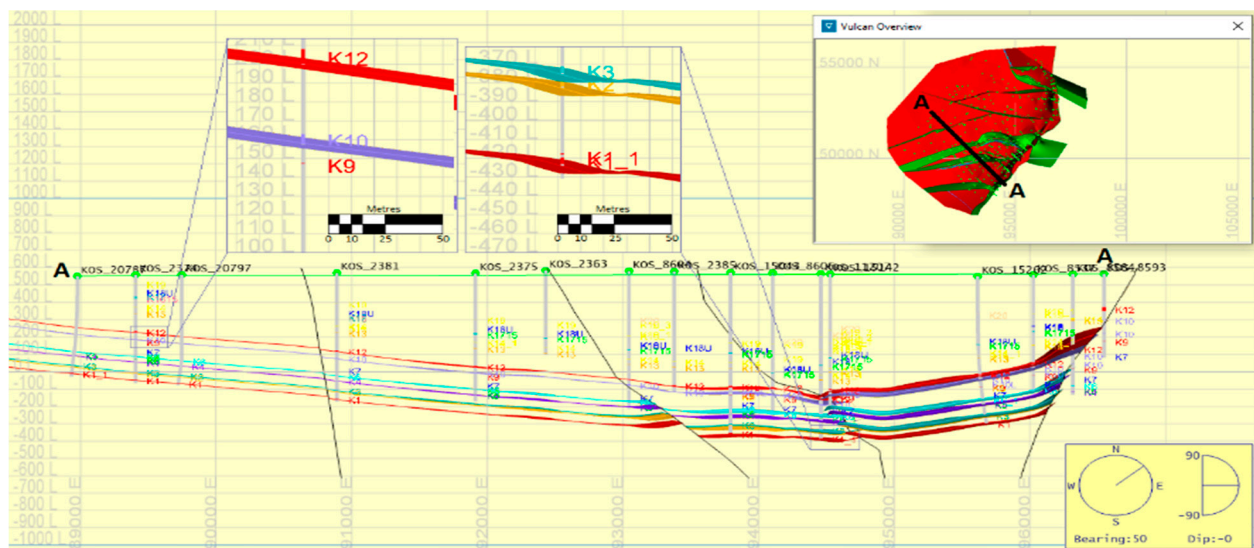
Figure 4. Cross-section of the floor surfaces of coal seams at Kostenko Mine along line A–A.
