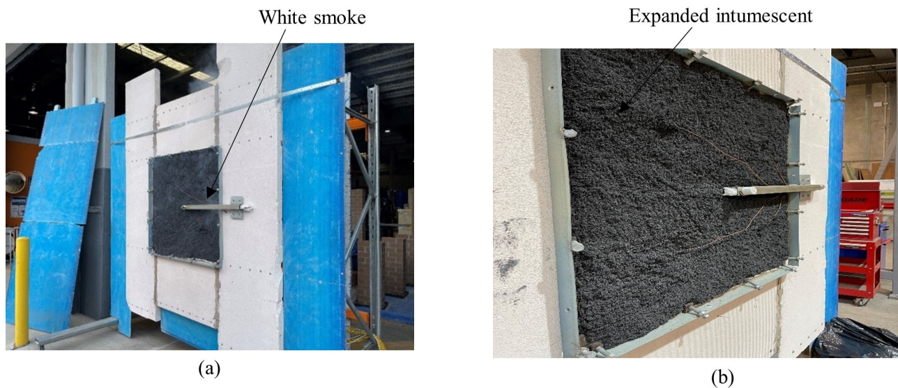
Figure 12. Test 4 specimen (a) during the test and (b) post-test.
