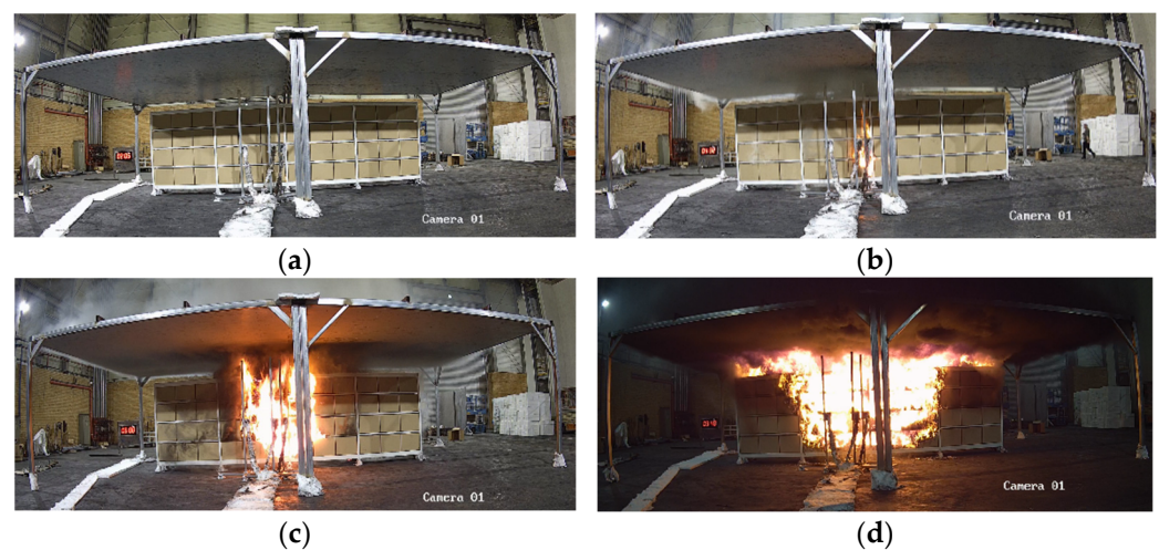
Figure 15. Combustion behavior over time. (a) Immediately after ignition; (b) 2 min 30 s after ignition; (c) 4 min after ignition; (d) 7 min 40 s after ignition.
