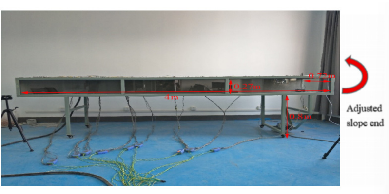
(a) Urban integrated common services tunnel model, 1:10th scale
