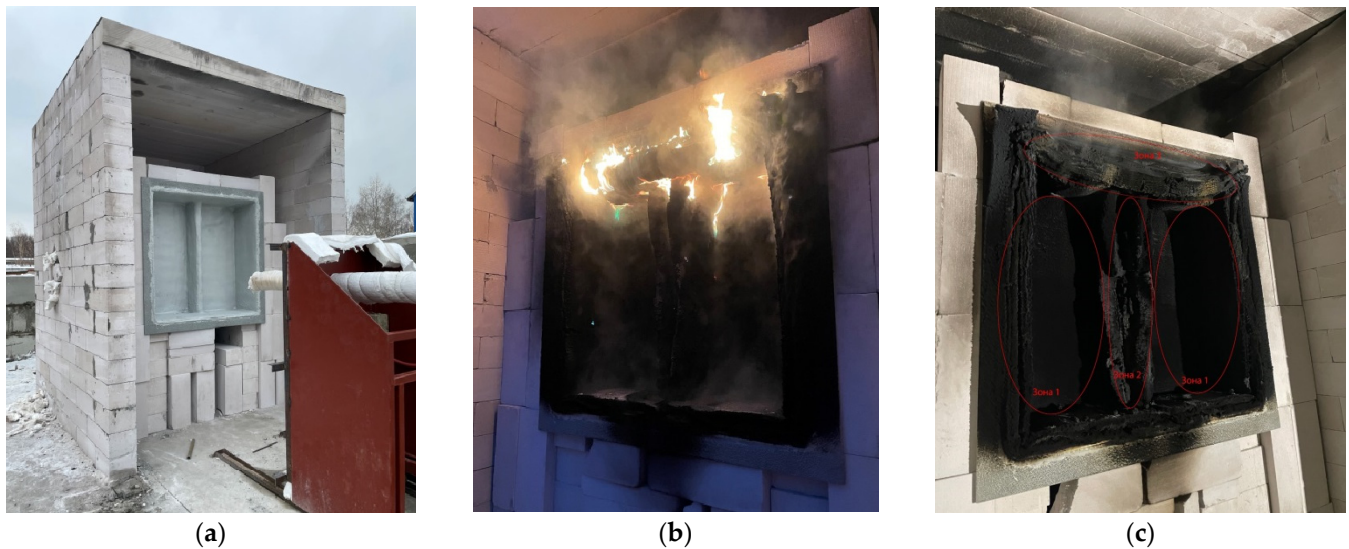
Figure 8. View of specimen No. 3: (a) before testing, (b) after testing, (c) after cooling.
