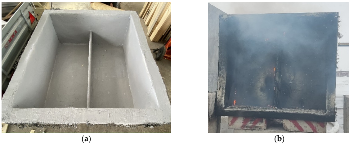
Figure 7. View of specimen No. 2: (a) before the test, (b) after the test.
