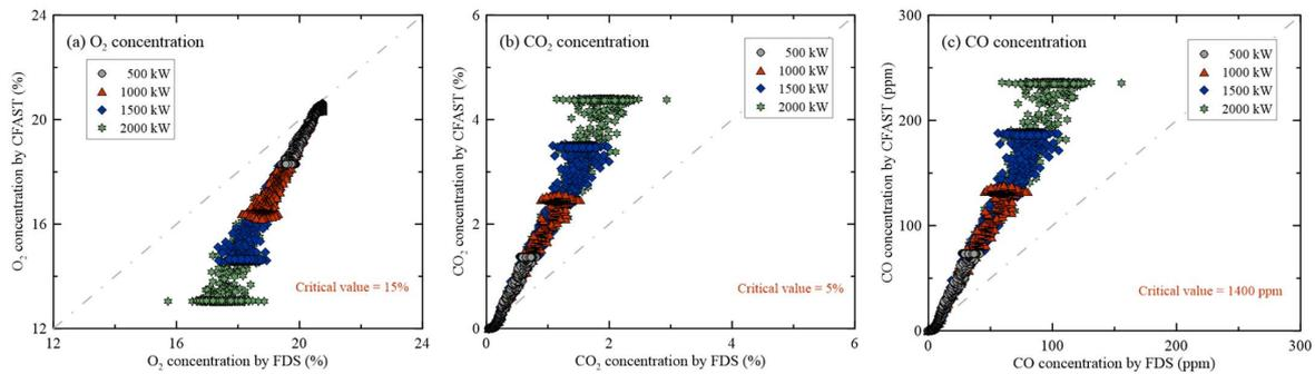
**Figure 6.** Comparison of O<sub>2</sub>, CO<sub>2</sub>, and CO concentrations based on the maximum HRR. (a) O<sub>2</sub> concentration; (b) CO<sub>2</sub> concentration; (c) CO concentration.
