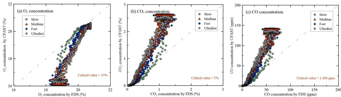
**Figure 5.** Comparison of  $O_2$ ,  $CO_2$ , and  $CO$  concentrations for different fire models against the fire growth rate. (a)  $O_2$  concentration; (b)  $CO_2$  concentration; (c)  $CO$  concentration.
