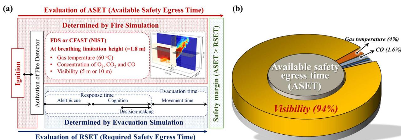
**Figure 1.** (a) Fire and evacuation simulation timeline for performance-based design (PBD) in building fires [8]; (b) Statistical proportions of the evaluation factors that determine the available safety egress time (ASET) [10].
