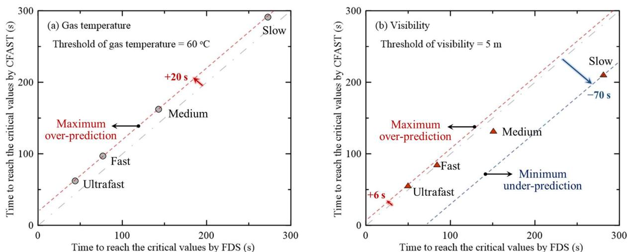
**Figure 10.** Comparison of the times needed to reach the critical value by FDS and CFAST. (a) Gas temperature; (b) Visibility.
