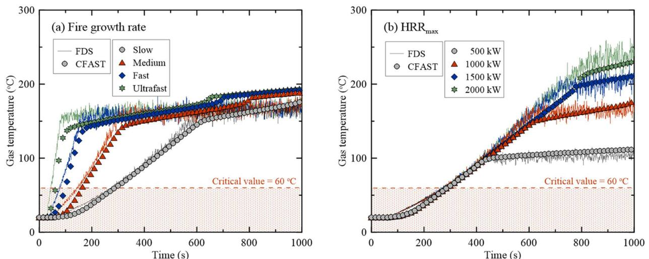
**Figure 8.** Comparison of the gas temperature using FDS and CFAST in terms of changes in the fire growth rate and maximum HRR. (a) Fire growth rate; (b)  $\text{HRR}_{\text{max}}$ .
