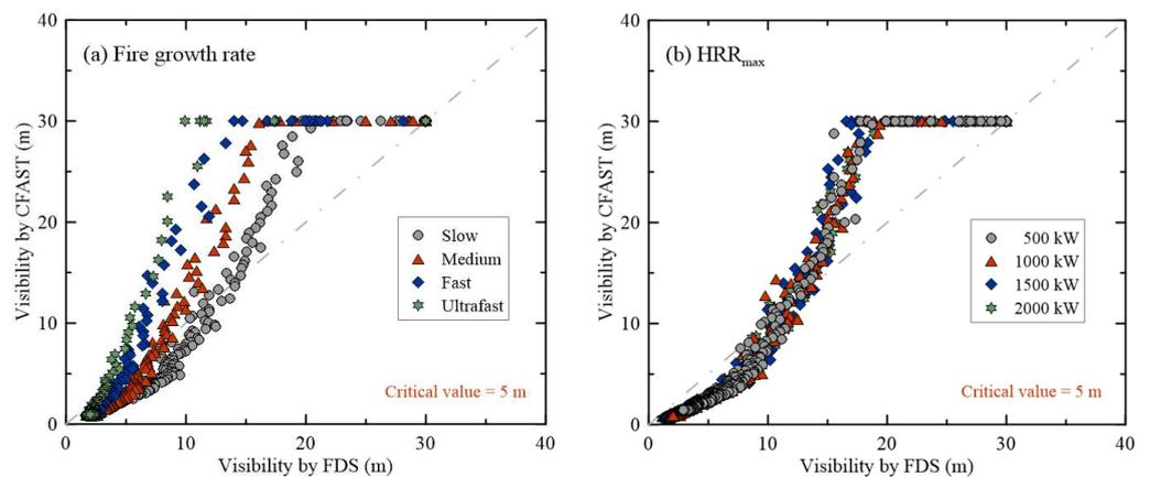
**Figure 7.** Comparison of visibility for the different fire models based on the fire growth rate and maximum HRR. (a) Fire growth rate; (b)  $HRR_{max}$ .
