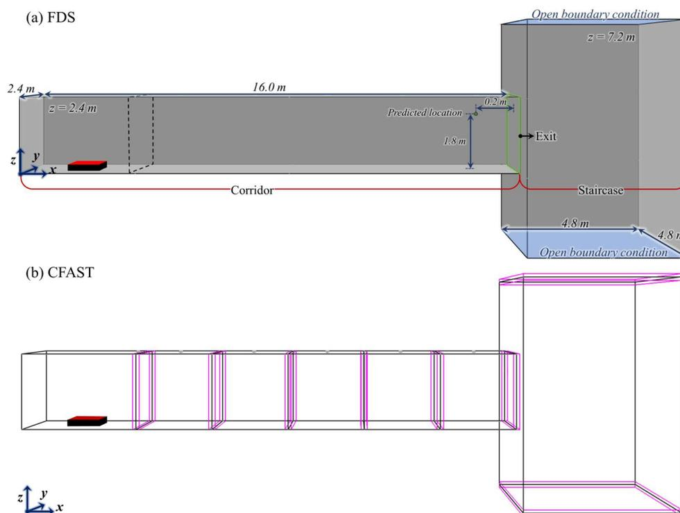
**Figure 2.** Schematic of the computational domain for the prediction of physical quantities related to the ASET. (a) FDS; (b) CFAST.
