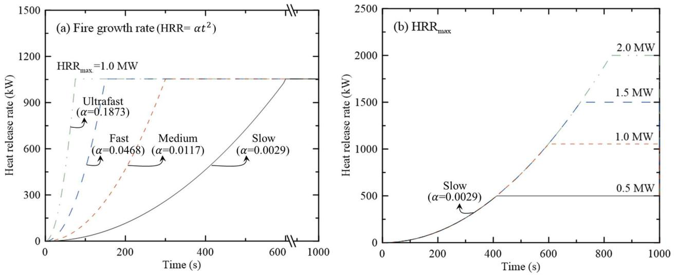
**Figure 3.** Fire conditions considered for the predictive performance comparison of the FDS and CFAST: (a) Fire growth rate (slow, medium, fast, and ultrafast); (b) Maximum heat release rate ( $HRR_{max}$ ).
