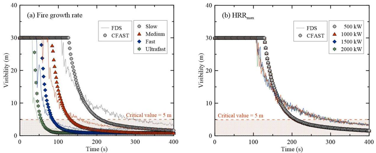
**Figure 9.** Comparison of visibility using FDS and CFAST regarding changes in the fire growth rate and maximum HRR. (a) Fire growth rate; (b)  $HRR_{max}$ .
