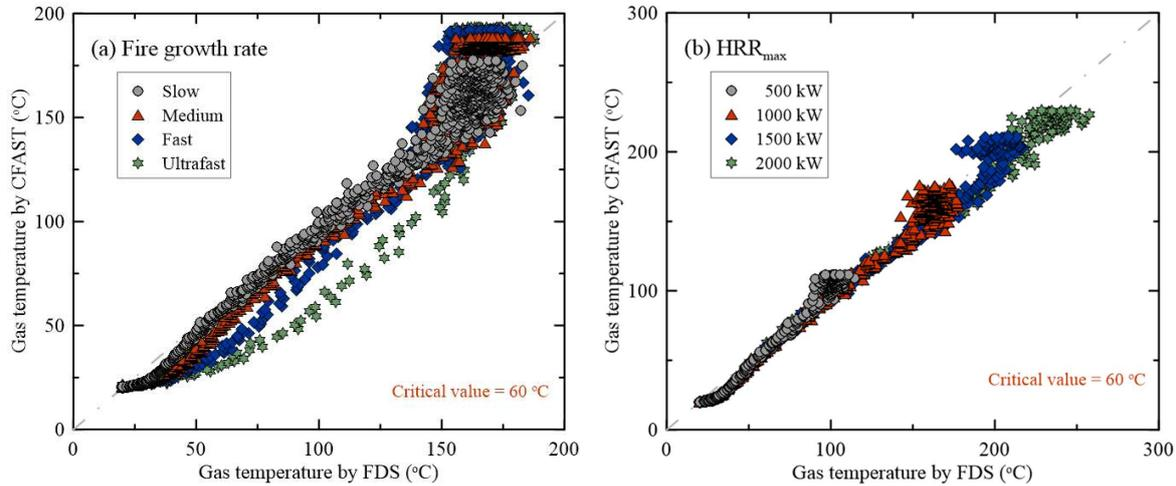
**Figure 4.** Comparison of gas temperatures for different fire models according to the (a) fire growth rate and (b) maximum heat release rate.
