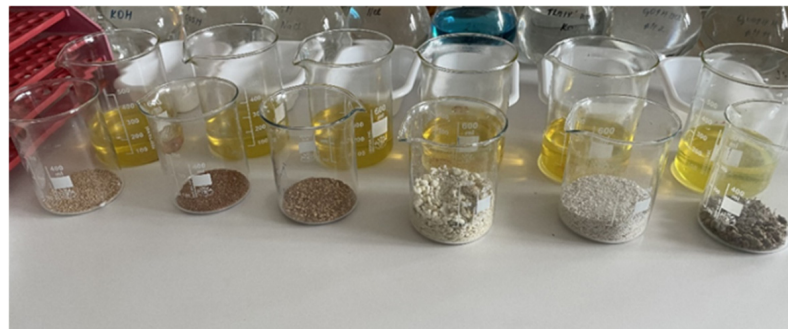
Figure 10. Measuring diesel fuel and determining the initial weight of the sorbent (source: elaborated by authors).
