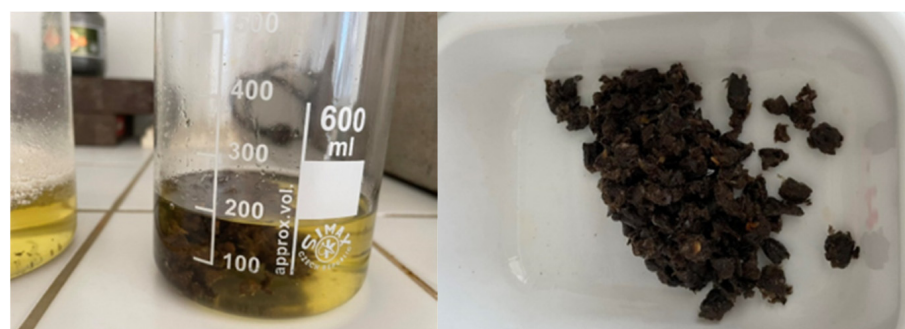
Figure 13. LITE-DRY immersed in gasoline and after draining (source: elaborated by authors).
