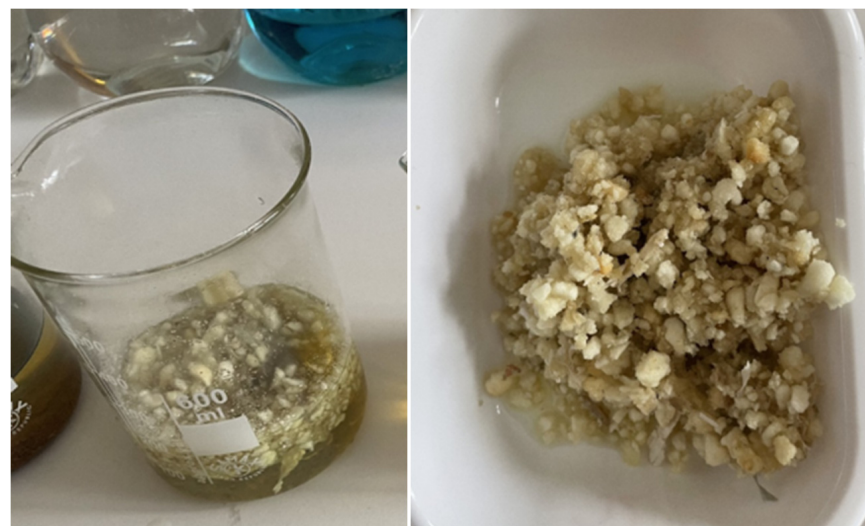
Figure 9. REOSORB immersed in diesel and after adsorption and dripping (source: elaborated by authors).
