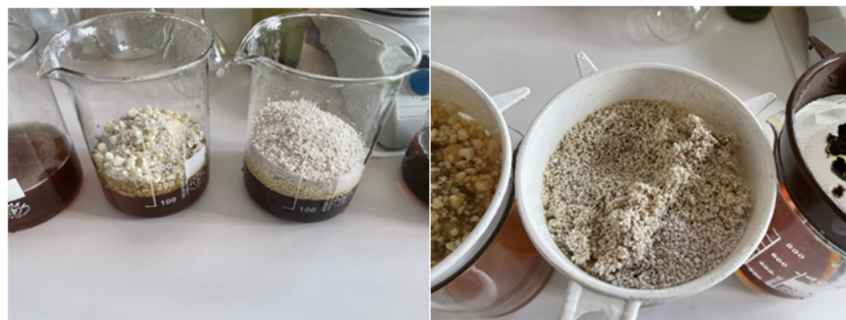
Figure 14. Vapex immersed in engine oil and after draining (source: elaborated by authors).
