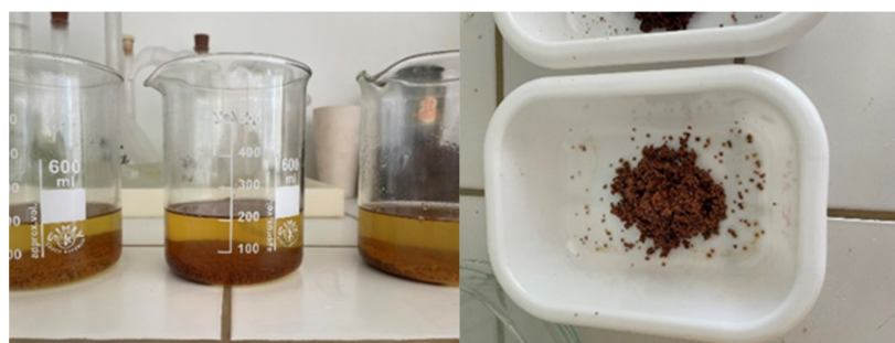
Figure 16. Absodan, Spilkleen, and ECO-DRY immersed in gasoline and ECO-DRY after dripping (source: elaborated by authors).
