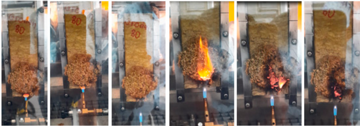
Figure 12. Different stages of ignition of dried Sagina Subulata SS embedded in mineral wool. Only the direct flame contact with the plant creates a flame front. After the flame is gone, the plant will not continue to burn. The embers gradually peter out.
