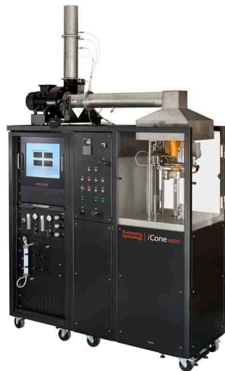
Figure 3. The FTT Dual Cone Calorimeter.
