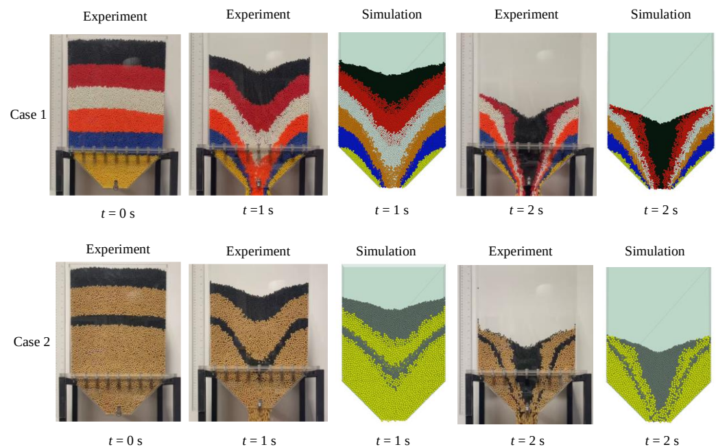
Figure 5. Comparison of flow patterns obtained from numerical simulation and experiments.
