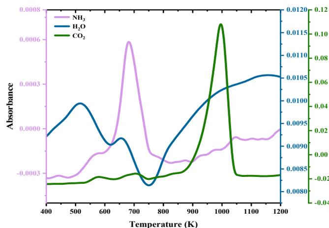
**Figure 3.** The evolution of main gaseous products at 10 K/min in nitrogen atmosphere.
