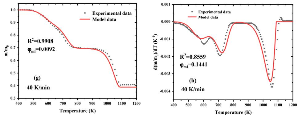
**Figure 7.** Estimated mass loss and mass loss rate based on the optimized parameters (lines) compared with experimental data (symbols): (a) mass loss at 10 K/min; (b) mass loss rate at 10 K/min; (c) mass loss at 20 K/min; (d) mass loss rate at 20 K/min; (e) mass loss at 30 K/min; (f) mass loss rate at 30 K/min; (g) mass loss at 40 K/min; (h) mass loss rate at 40 K/min.
