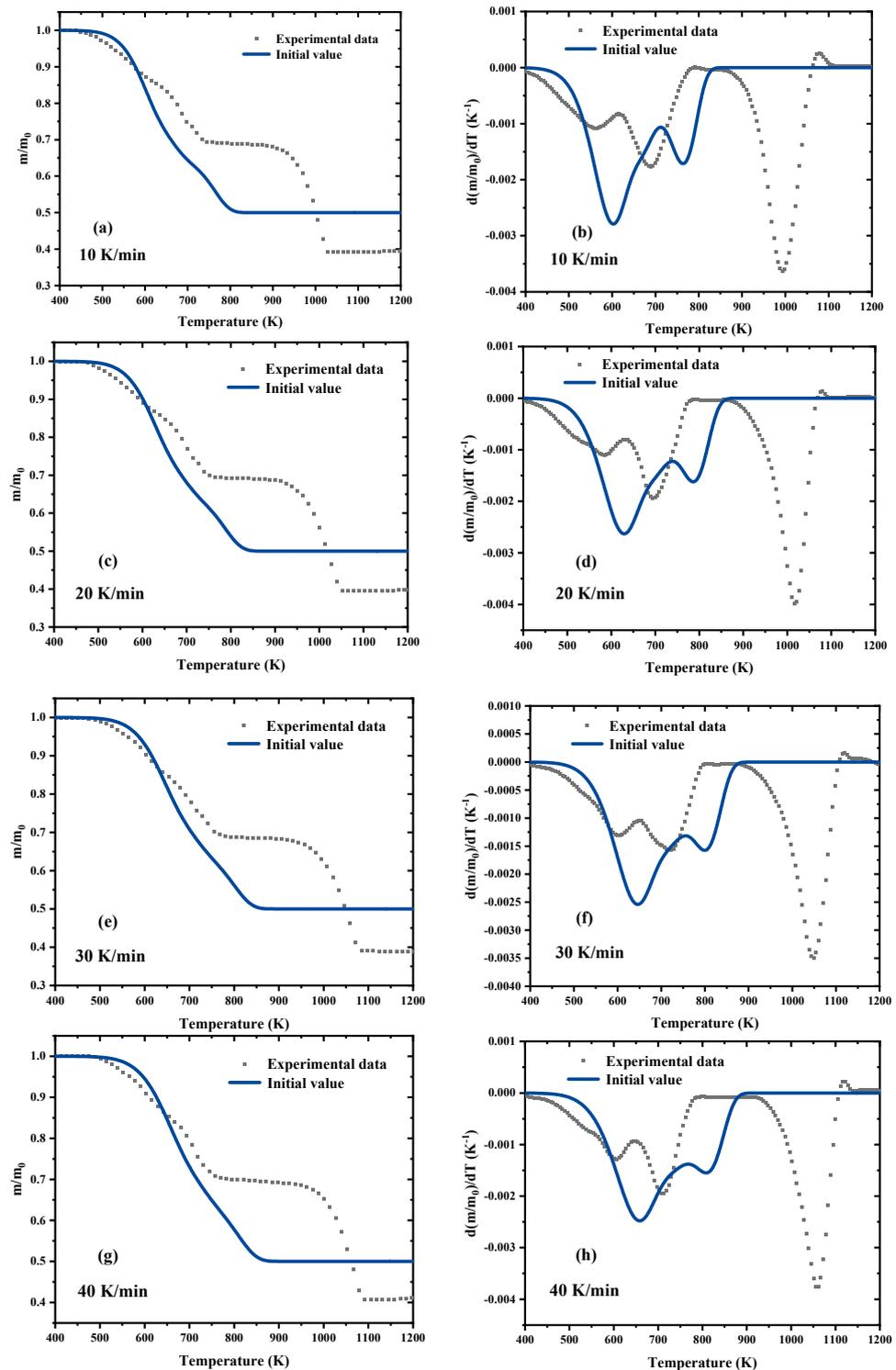
**Figure 6.** Experimental data (symbols) compared to estimated results (lines) based on the initial parameters values: (a) mass loss at 10 K/min; (b) mass loss rate at 10 K/min; (c) mass loss at 20 K/min; (d) mass loss rate at 20 K/min; (e) mass loss at 30 K/min; (f) mass loss rate at 30 K/min; (g) mass loss at 40 K/min; (h) mass loss rate at 40 K/min.
