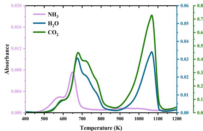
**Figure 5.** The evolution of main gaseous products at 10 K/min in air atmosphere.
