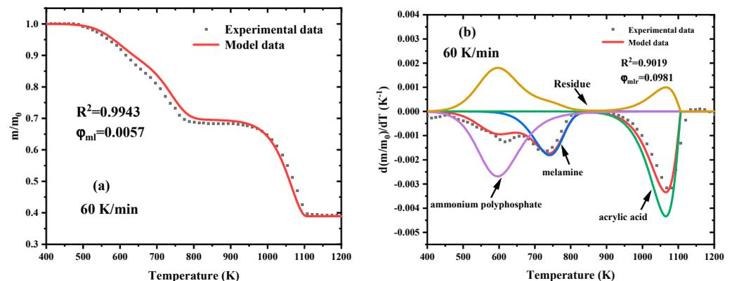
**Figure 8.** Estimated mass loss and mass loss rate based on the optimized parameters at 60 K/min: (a) mass loss; (b) mass loss rate.
