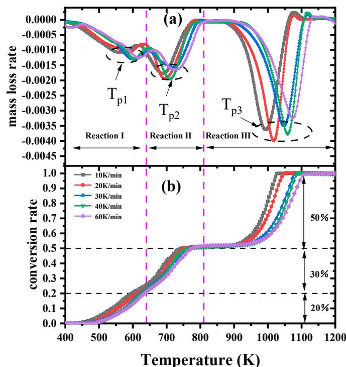
**Figure 1.** Mass loss rate and conversion rate of fireproof sealant at various heating rates: (a) mass loss rate; (b) conversion rate.
