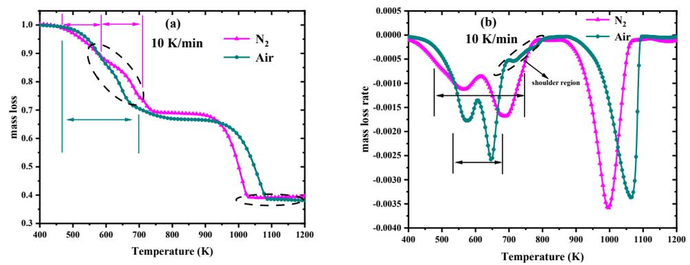
**Figure 4.** Comparison of mass loss and mass loss rate of fireproof sealant at 10 K/min in nitrogen and air atmosphere: (a) mass loss; (b) mass loss rate.
