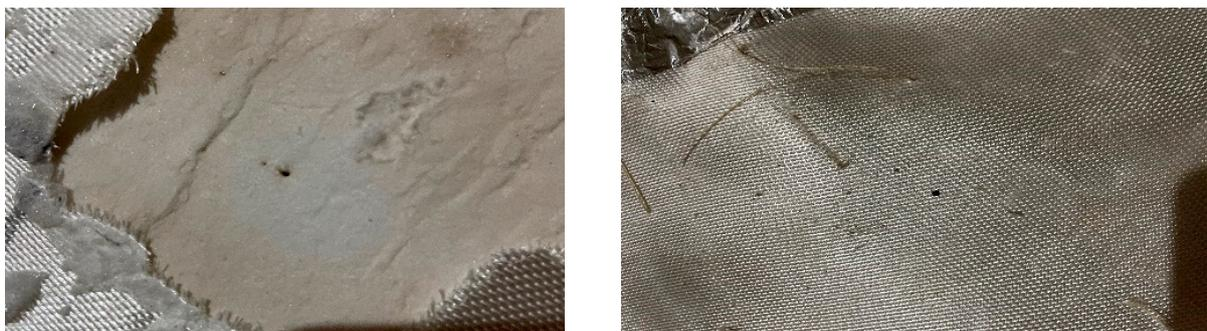
**Figure 14.** Occurrence of breakdowns on Sample No. 7 in a small-scale test under standard temperature conditions.
