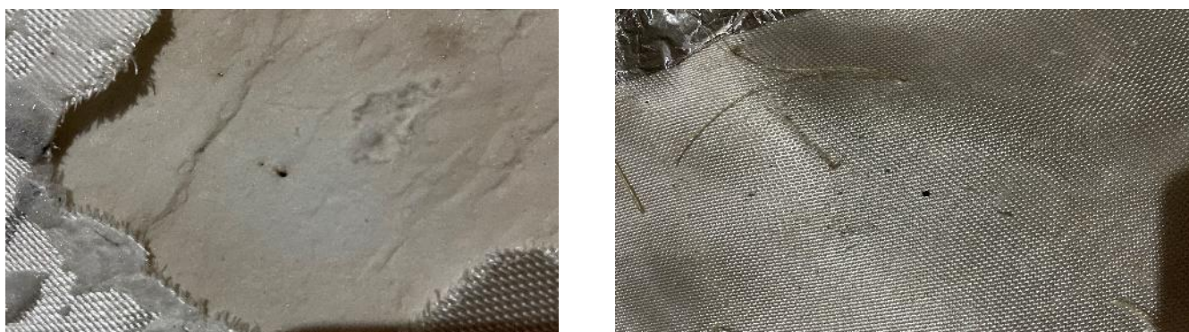
Figure 14. Occurrence of breakdowns on Sample No. 7 in a small-scale test under standard temperature conditions.
