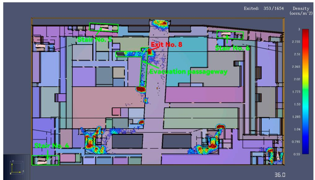
Figure 29. Evacuation simulation result at 36 s.
