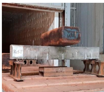
(a) Service load of 25 kN
