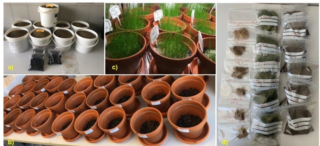
Figure 3. (a) Burnt soil with soil amendments before mixing; (b) terracotta pots; (c) Lolium perenne biomass growth; (d) dried and packed AGB, UGB, and soil after pot experiment.
