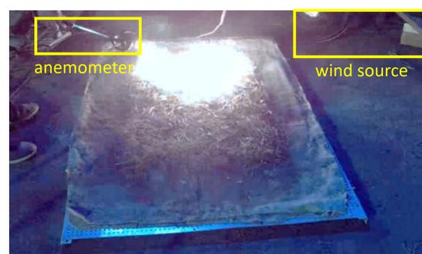
**Figure 9.** Burning experiment configuration. The picture shows a hand-held anemometer in the upper-left corner and a wind source in the upper-right corner.
