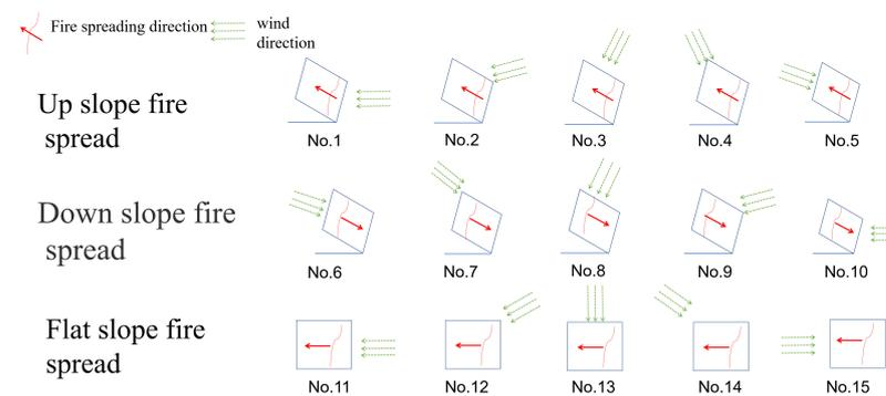
**Figure 8.** Fifteen kinds of fire spread experiments. Three types of slope. Five kinds angle between fire spread direction and wind direction. From left to right, the angle between the wind direction and fire spread direction is 0°, 45°, 90°, 135°, and 180°.
