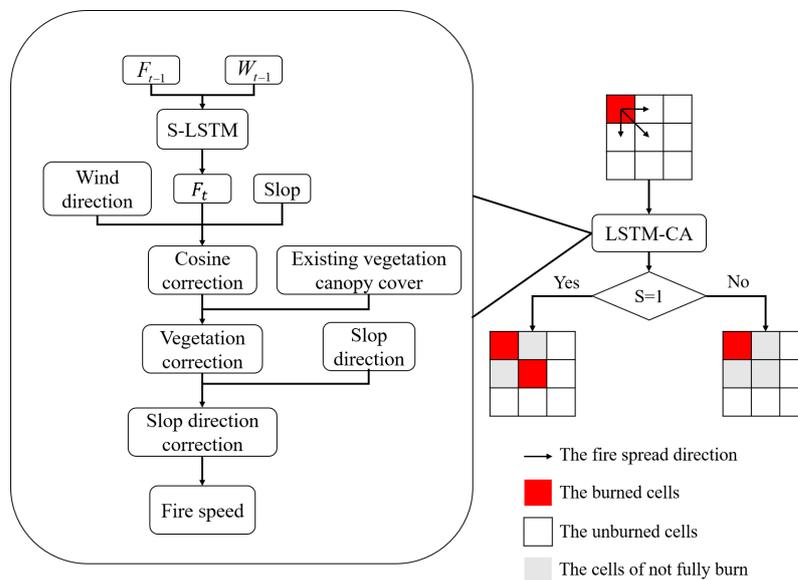
**Figure 5.** The framework of the LSTM-CA model.
