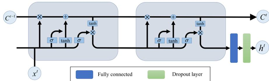
**Figure 2.** The LSTM cell structure.  $x^t$  and  $h^t$  are both one-dimensional matrices composed of wind speed and the ROS.
