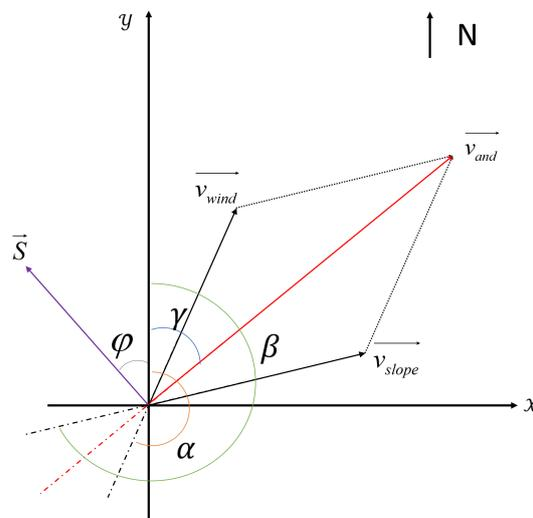
**Figure 6.** Wind direction and slope vector diagram.  $\alpha$  is the angle of wind direction,  $\beta$  is the angle of slope direction,  $\gamma$  is the angle of main direction, and  $\varphi$  is the angle between the spread direction ( $\vec{S}$ ) and the positive direction of the y-axis.
