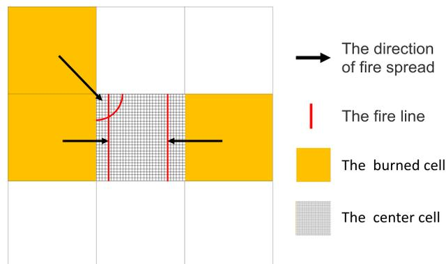
**Figure 7.** Example of fire spreading from the eight directional cells to the central cell. The adjacent cells spread to the central cell in a rectangle, and the sub-adjacent cells spread to the central cell in a quarter circle.
