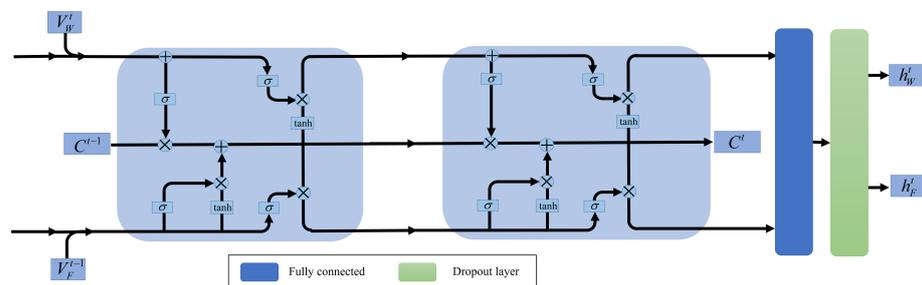
**Figure 3.** The S-LSTM cell structure. The ROS ( $V_F^t$ ) and wind speed ( $V_W^t$ ) as input to the S-LSTM model, respectively.
