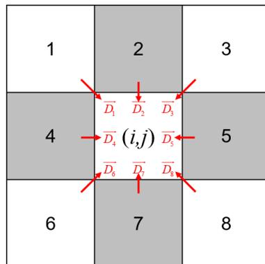
**Figure 4.** Moore-neighbourhood type of two-dimensional CA. The cells of 2, 4, 5, and 7 are adjacent cells. The cells of 1, 3, 6, and 8 are sub-adjacent cells.  $\vec{D}_i$  denotes the direction from the  $i$ -th cell to the central cell.
