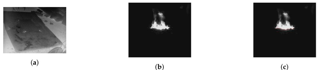
**Figure 10.** The extraction process of the infrared image fire line. (a) is an infrared image with four calibration points, (b) is the image after perspective transformation, and (c) is the infrared image with the fire line.
