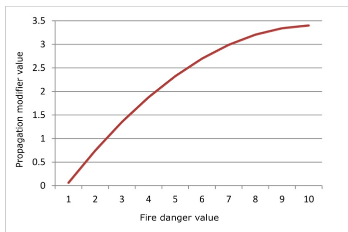
Figure S1. The propagation value curve as a function of the fire danger value setting.
