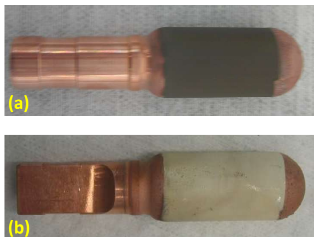
Figure 34. The high-voltage contact fingers silver-coated by LTPS (a) directly after coating and (b) after reduction. The plasma jet reduction was conducted with PB3 operated at 55 mbar with a gas mixture of 95% nitrogen + 5% hydrogen with flow rate of 55 SLM, pumping speed of 105 m 3 h −1 , and treatment time of 40 s. Internal report of Reinhausen Plasma GmbH.
