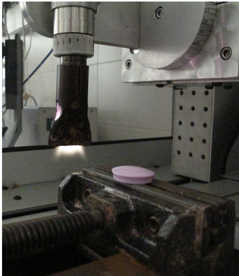
Figure 28. The prototype nozzle extension for PB3, allowing for the widening of the plasma plume up to 80 mm. Internal report of relyon plasma GmbH.
