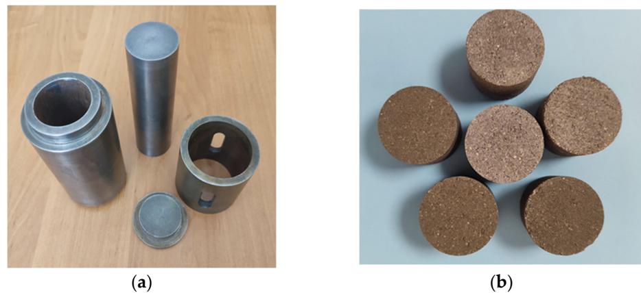
Figure 2. Pictures of the pressing mold (a) and formed samples (b).
