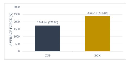
Figure 5. Bar chart for the average fracture strength of CAD/CAM materials in zirconia dioxide.
