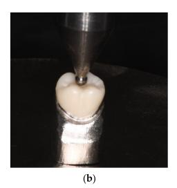
**Figure 3.** (a) Master die in cast metal. (b) Load of the punch in tempered steel on the sample seated in the cast metal die.
