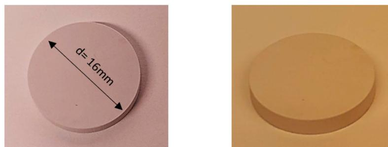
**Figure 8.** AlN-sample-discs (two views) based on suspension with 46 vol% solid content, green state.
