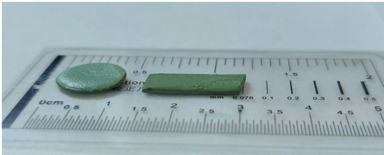
**Figure 6.** Printed samples of NiO/YSZ anodes of various shapes on a calibration ruler.
