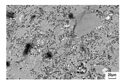
**Figure 7.** SEM image of ceramic paste texture with evidence of developed vitrification. The magnification  $368 \times$ .
