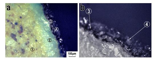
**Figure 5.** The OM image of the sample's profile section showing layers sequence. (a): 1—the paste, 2—white slip, 3—black glaze, 4—transparent glaze. (b): 3—black glaze, 4—transparent glaze. The magnification  $50\times$ .
