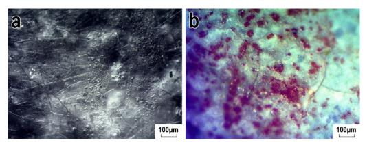
**Figure 9.** OM images of surface texture of the black area (**a**) and red area (**b**) on the separate fragment of the figurine. The magnification is  $50 \times$ .
