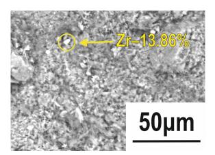
Figure 8. SEM image of the spectral surface with the indicated location of the zirconium inclusion.
