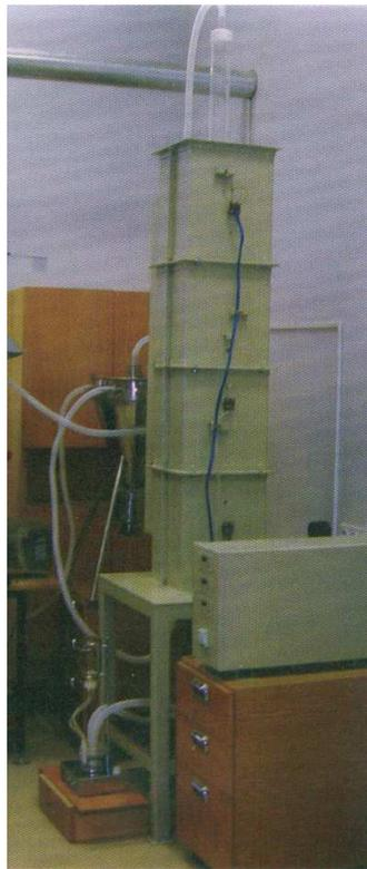
**Figure 2.** General view of a laboratory equipment for the synthesis of aerosol powders by ultrasonic spray pyrolysis.
