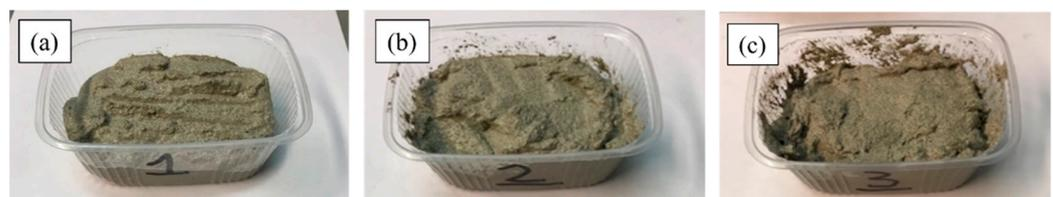
**Figure 2.** Samples of the Thermacoat™ powder mixed with water (a), with 2.5 wt.% excess addition of cenospheres (b) and 1 wt.% polypropylene fibers (c).
