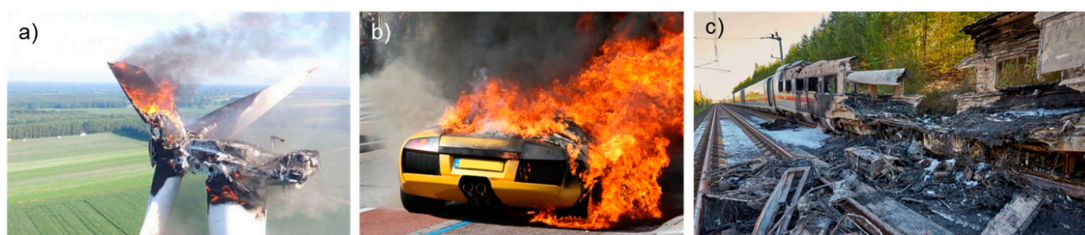
Figure 1. Fire of Polymer Matrix Composites (PMC) components with low thermal resistivity: (a) Wind turbine [2]; (b) Lamborghini Murcielago [3]; (c) Intercity-Express high speed train [4].
