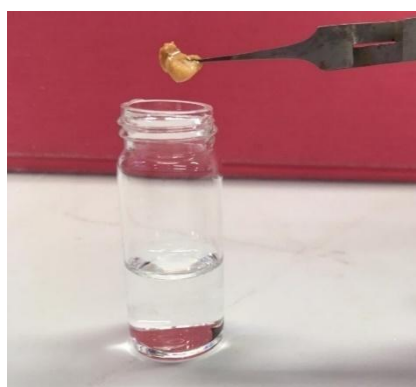
Figure S12. The photo shows the glutaraldehyde-crosslinked CM/UiO-66-1 monolith can be easily picked up after six hours immersed in MCPP solution.
