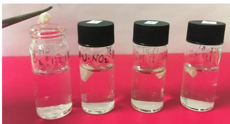
Figure S9. The photo shows the stability of the base-treated composite monoliths with UiO-66-NO 2 or UiO-66-NH 2 after adsorption testing; immersed in 10 mL of 60 ppm MCP solution for 6 h. From left to right: CM/UiO-66-NO 2 -2, CM/UiO-66-NO 2 -1, CM/UiO-66-NH 2 -2, CM/UiO-66-NH 2 -1.
