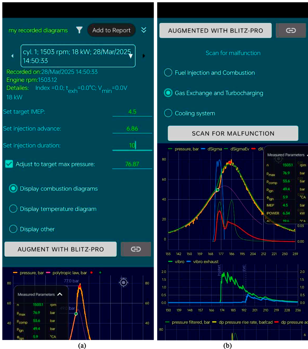
Figure 16. Screenshots of the DEPAS 5.0W Android application illustrating the implementation of the digital twin for (a) augmenting diagnostic data with digital twin simulation results and (b) optional further analysis for possible malfunctions.
