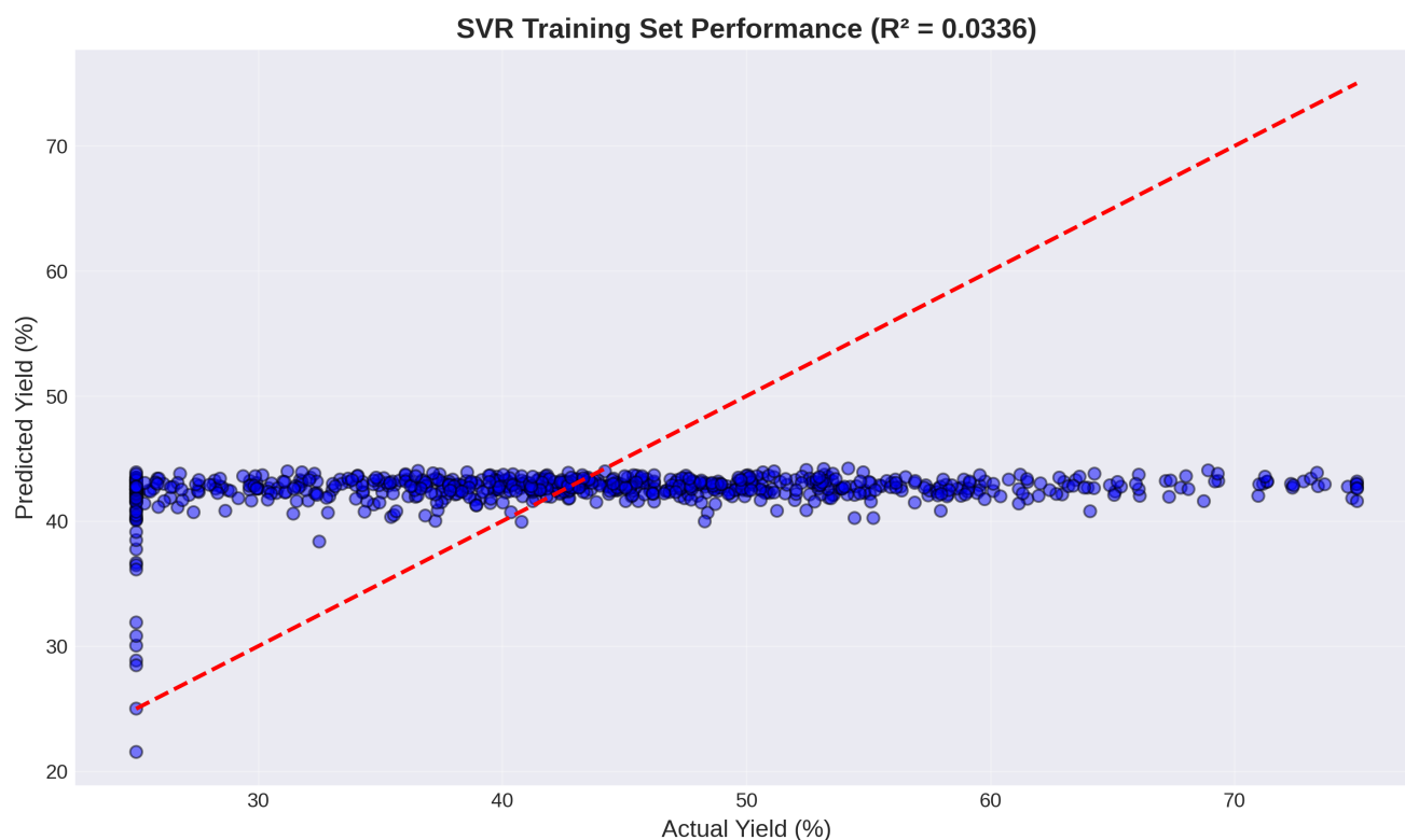
Figure 7. SVR training set performance ( R^2 = 0.0336 ). The scatter plot shows actual versus predicted production yield, with wide dispersion of points around the ideal diagonal. The red dotted line represents the ideal reference line ( y = x ), indicating perfect prediction.
