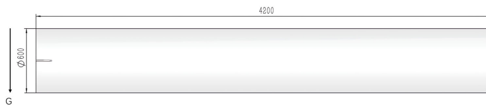
Figure 8. Fluid simulation model setup (Single Nozzle).
