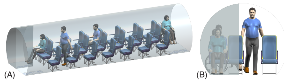
Figure 10. Rendering of a pod with maximum packaging for 21 passengers plus one person with reduced mobility in an isometric view (A) and front view (B).
