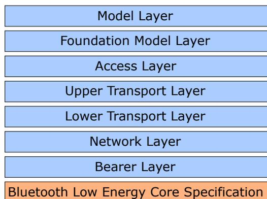
**Figure 1.** Bluetooth Mesh Profile stack.
