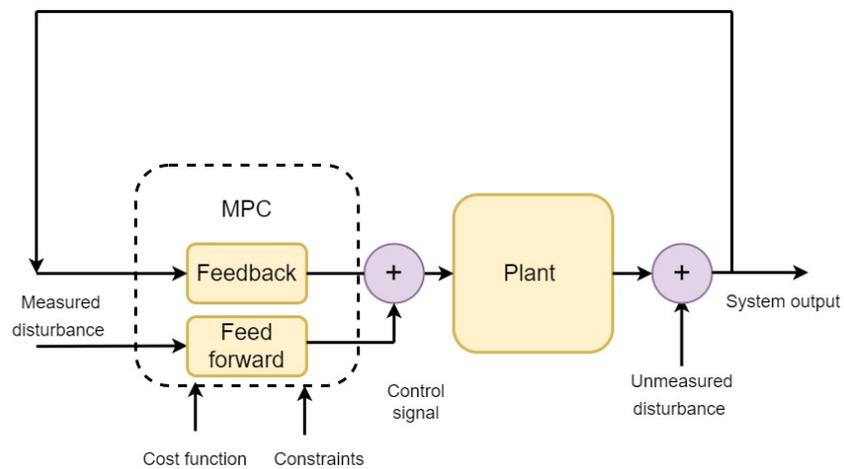
Figure 8. Feedback and feedforward MPC [55].
