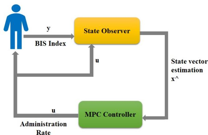
**Figure 9.** NMPC closed-loop structure in anaesthesia.
