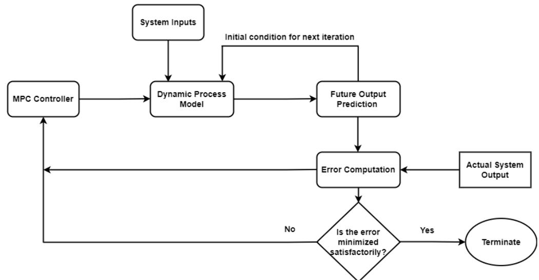
**Figure 4.** Generalized MPC tuning methodology.
