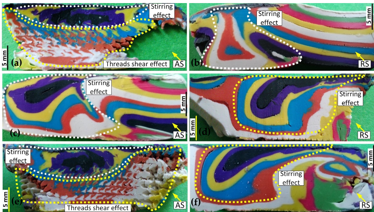
Figure 7. The cross-sections of the stirring zone showing the internal flow details for the plasticine analogue sample; (a,b) cross-sections of the entry zone; the advancing side (AS) and retreating side (RS) transverse sections, respectively; (c,d) cross-sections of the mid-weld; the AS and RS transverse sections, respectively; (e,f) cross-sections of the exit zone; the AS and RS transverse sections, respectively.
